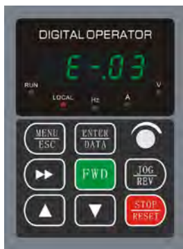
Fig. 4-5 Fault alarm display state
