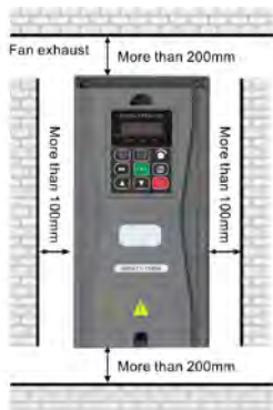
Figure 3-1 Mounting space and distance
